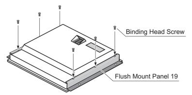
Note: Attach the flush mount panels to both sides of the monitor unit with no gap.
